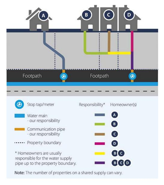
If the pipe is in poor condition, we recommend you and your neighbours replace it with separate pipes. This would improve both the flow and the pressure of water at your tap. We can require separation of a shared pipe in certain circumstances:
